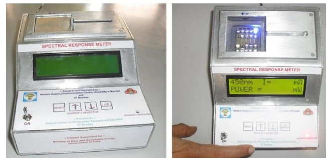
Fig.1. An experimental setup to measure the spectral response and external quantum efficiency of mono-Si solar cell [17].
