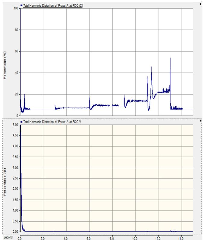
Fig. 14. THD for Current and Voltage
