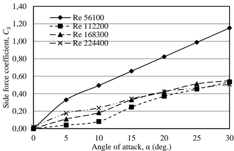
Fig. 11. Side force coefficients for racing bike without wind turbine.
