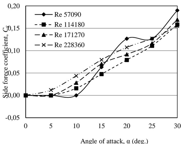
Fig. 14. Side force coefficients for racing bike with wind turbine.
