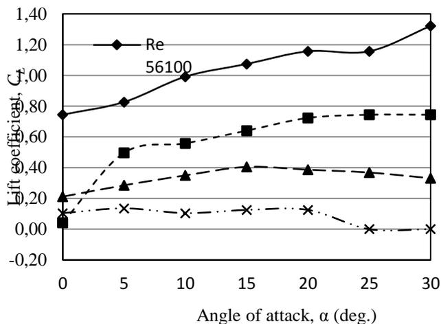
Fig. 8. Lift coefficients for racing bike with wind turbine
