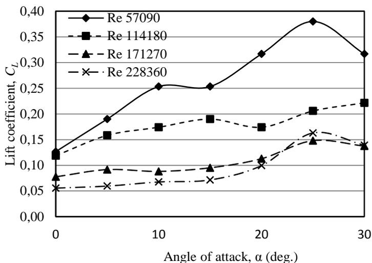
Fig. 10. Lift coefficients for dirt bike with wind turbine
