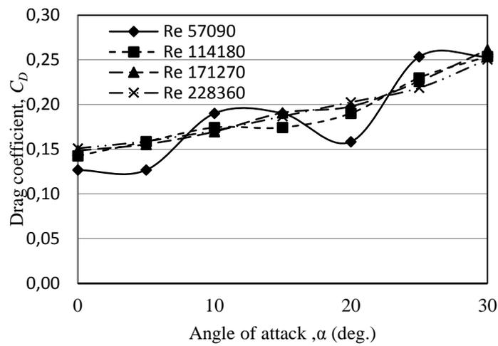
Fig. 5. Drag coefficients for dirt bike without wind turbine
