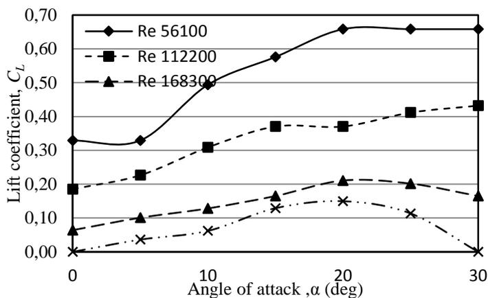
Fig. 7. Lift coefficients for racing bike without wind turbine
