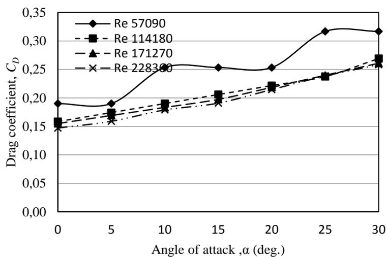
Fig. 6. Drag coefficients for dirt bike with wind turbine
