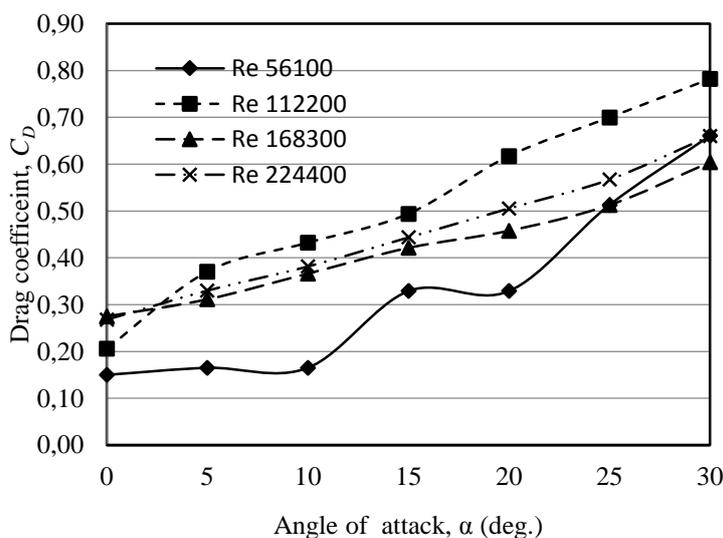
Fig. 3. Drag coefficients for racing bike without wind turbine
