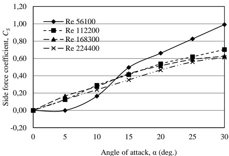
Fig. 12. Side force coefficients for racing bike with wind turbine
