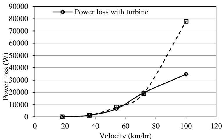
Fig. 17. Power loss for dirt bike.
