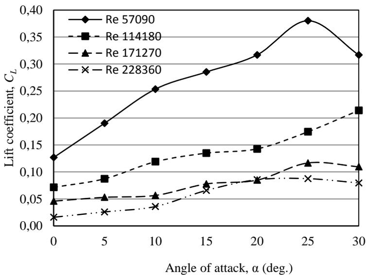
Fig. 9. Lift coefficients for dirt bike without wind turbine
