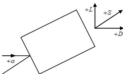
**Fig. 2.** Positive directions of angle of attack and aerodynamic forces.
