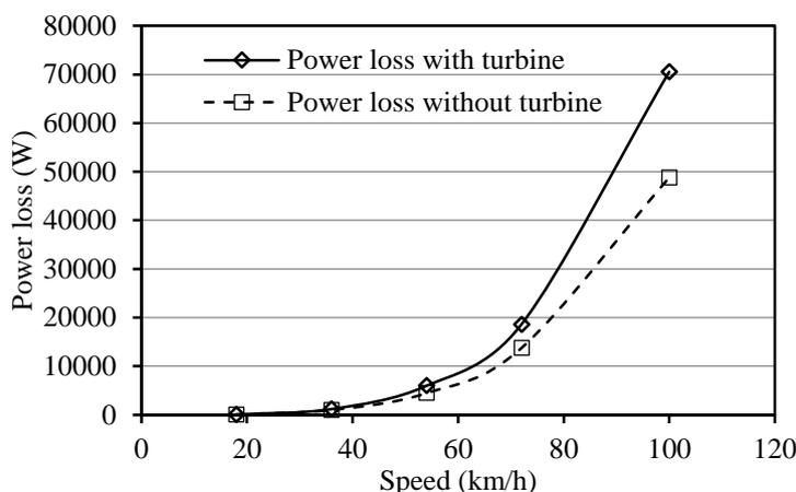
Fig. 16. Power loss for racing bike.
