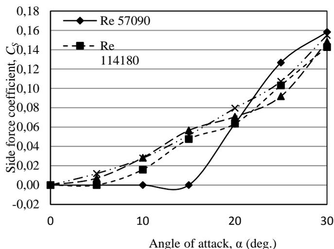
Fig. 13. Side force coefficients for dirt bike without wind turbine.
