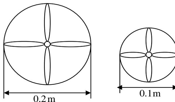
Fig. 15. The selected diameter of the wind turbine propeller.
