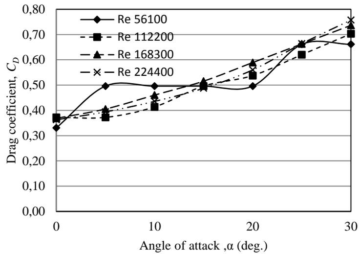
Fig. 4. Drag coefficients for racing bike with wind turbine
