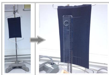
Figure 2. The placement of the specimen to the test apparatus [34].
