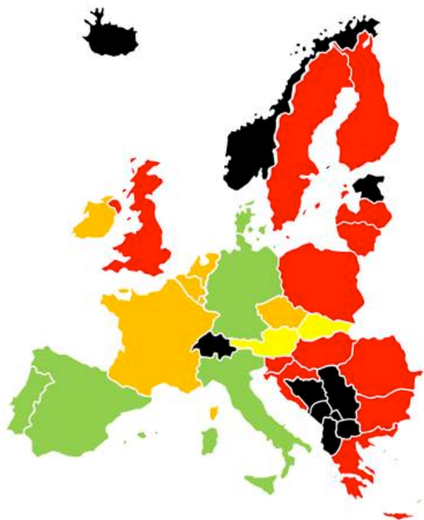
Figure 4. Comparing LCOE (VAT included) with the actual electricity price in the various member state of the Union. In green the countries where grid parity for small PV residential plants has been already reached, red marks the opposite situation while yellow and orange represent situation where differences within 10% and 20% respectively, can be found
