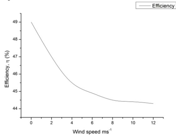
**Fig. 6.** Variation of efficiency with wind speed
