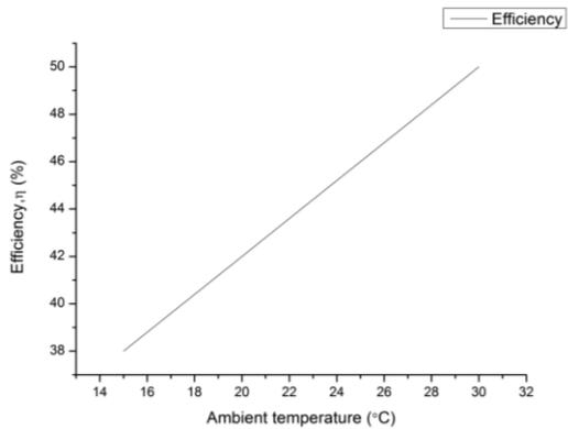
**Fig. 4.** Influence of ambient temperature on the system efficiency
