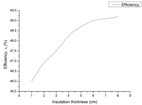
**Fig. 5.** Effect of insulation thickness on the system efficiency
