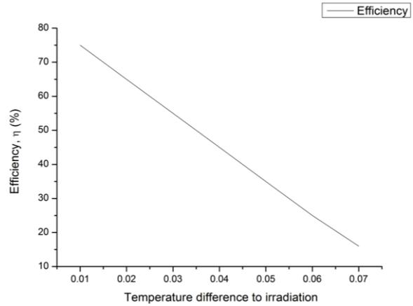
Fig. 9. Variation of efficiency with ratio of temperature difference to the solar radiation
