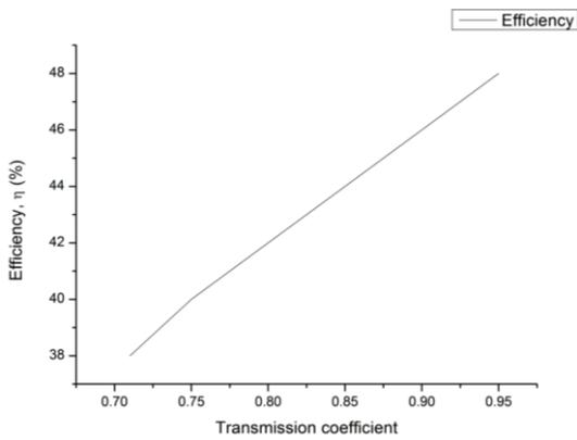
Fig. 7. Effect of transmission coefficient of the glass cover .
