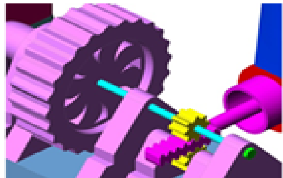
Fig. 15. Gear mechanism of proposed conversion system
