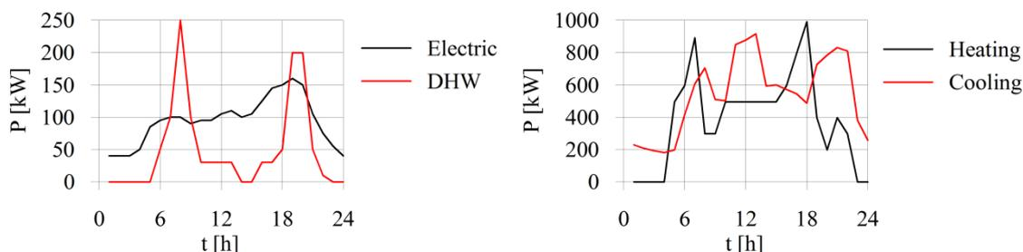
**Fig. 3.** User electric and DHW (on the left) and heating and cooling (on the right) hourly demand.
