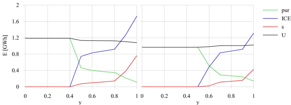
**Fig. 9.** Annual balance of the electrical energy for Case 1 (on the left) and Case 2 (on the right).
