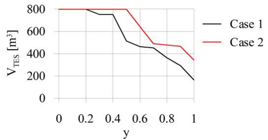
**Fig. 7.** TES volume as a function of the parameter  $y$ .
