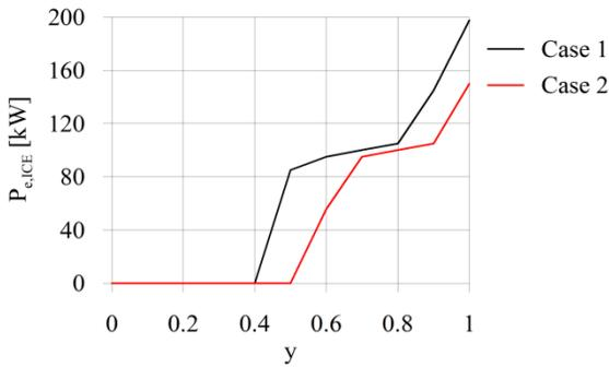
**Fig. 4.** ICE size as function of the parameter  $y$ .
