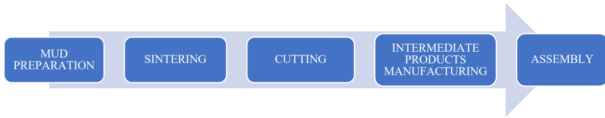
Figure 2. Medium voltage fuse production flow chart
