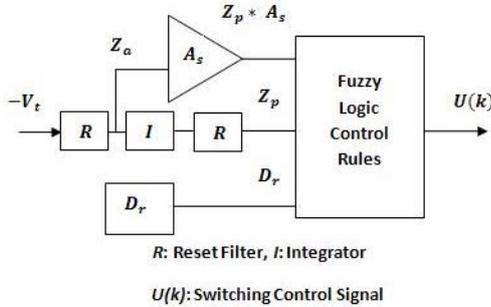
Fig. 6. Fuzzy Logic Switching Controller
