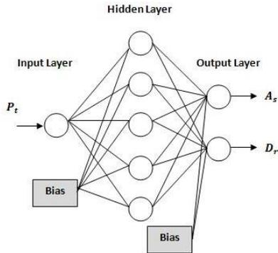
Fig. 7. Configuration of Artificial Neural Network
