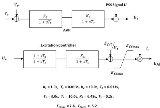
**Fig. 2.** Conventional excitation control system for Unit 1 and Unit 4
