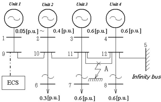
**Fig. 1.** A Longitudinal four-machine infinite bus system
