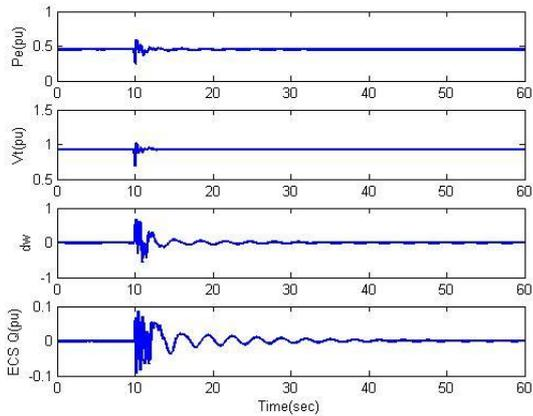
**Fig. 9.** Voltage profile of bus 9, power flow of infinite bus, speed deviation of Unit 1 of the system on Fig. 2 with ECS control operation (Setting of Power Output from Unit 1 = 0.5 pu and  $Q_{smax}=0.05$ puMVar).
