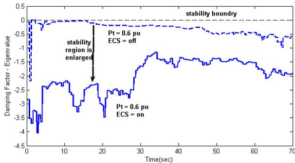
**Fig. 12.** Eigenvalue based stability evaluation of the study system. (Dashed and solid lines show the cases of ECS is off and on respectively)
