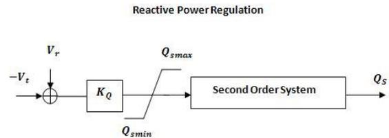
**Fig. 5.** Basic Configuration of mathematical model for ECS
