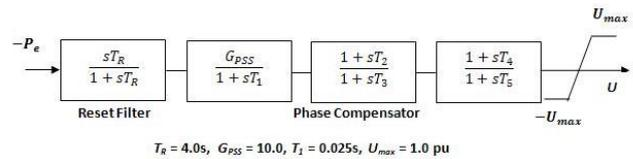
**Fig. 4.** Conventional power system stabilizer (CPSS)
