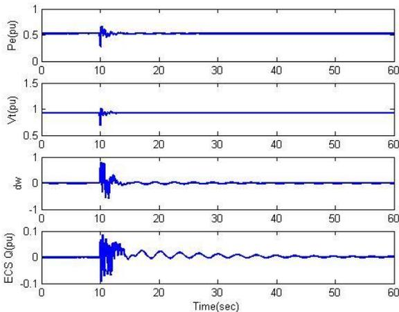
**Fig. 10.** Voltage profile of bus 9, power flow of infinite bus, speed deviation of Unit 1 of the system on Fig. 2 with ECS control operation (Setting of Power Output from Unit 1 = 0.6 pu and  $Q_{smax}=0.05$ puMVar).
