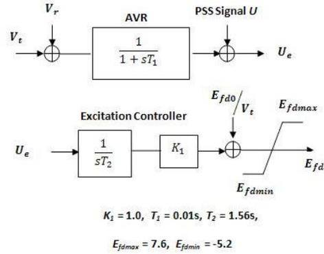
**Fig. 3.** Conventional excitation control system for Unit 2 and Unit
