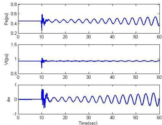
Fig. 8. Voltage profile of bus 9, power flow of infinite bus, speed deviation of Unit 1 of the system on Fig. 2 without
