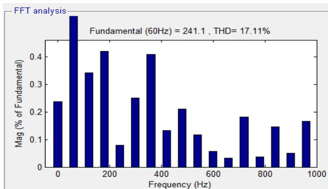
Fig. 13. THD of Vab voltage for one cycle
