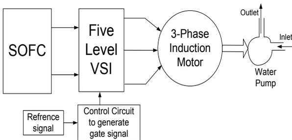
**Fig. 1.** Schematic diagram of complete system
