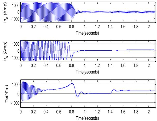
**Fig. 9.** Stator current, rotor current and Electromagnetic torque
