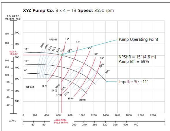
Fig. 5. Pump performance curve
