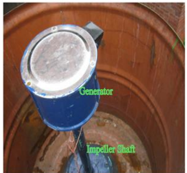
Fig 7. Inside view of the drum which is mounted upper where generator and impeller shaft are seen
