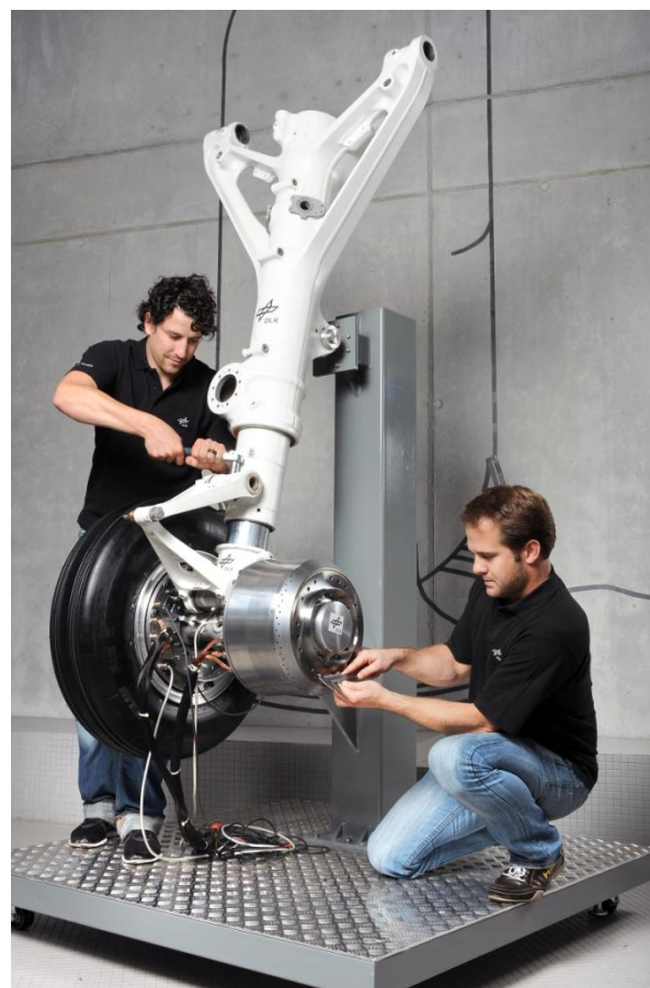
Fig.21. Nose leg gear with the electric wheel hub motor for autonomous taxiing of a passenger aircraft Airbus A320
