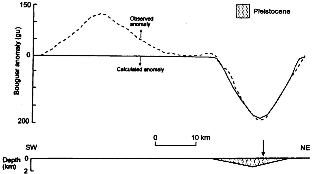
Figure 10. Interpreted two-dimensional gravity anomaly profile AA' shown in Figure 3 including only the Kızılırmak River Basin. Arrow shows the location of the Kızılırmak river.
