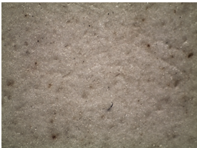
Figure 4. Microscopic image of a vacuum mixed sample.
