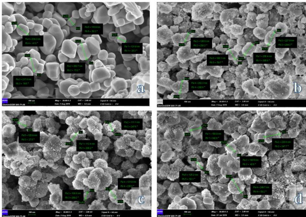
Figure 5. Particle size representation of a) pure TiO<sub>2</sub> b) TiO<sub>2</sub>+ sodium dodecyl sulfate (SDS) c) TiO<sub>2</sub>+cetyl trimethyl ammonium bromide (CTAB), and d) TiO<sub>2</sub>+nonionic (TritonX-100).
