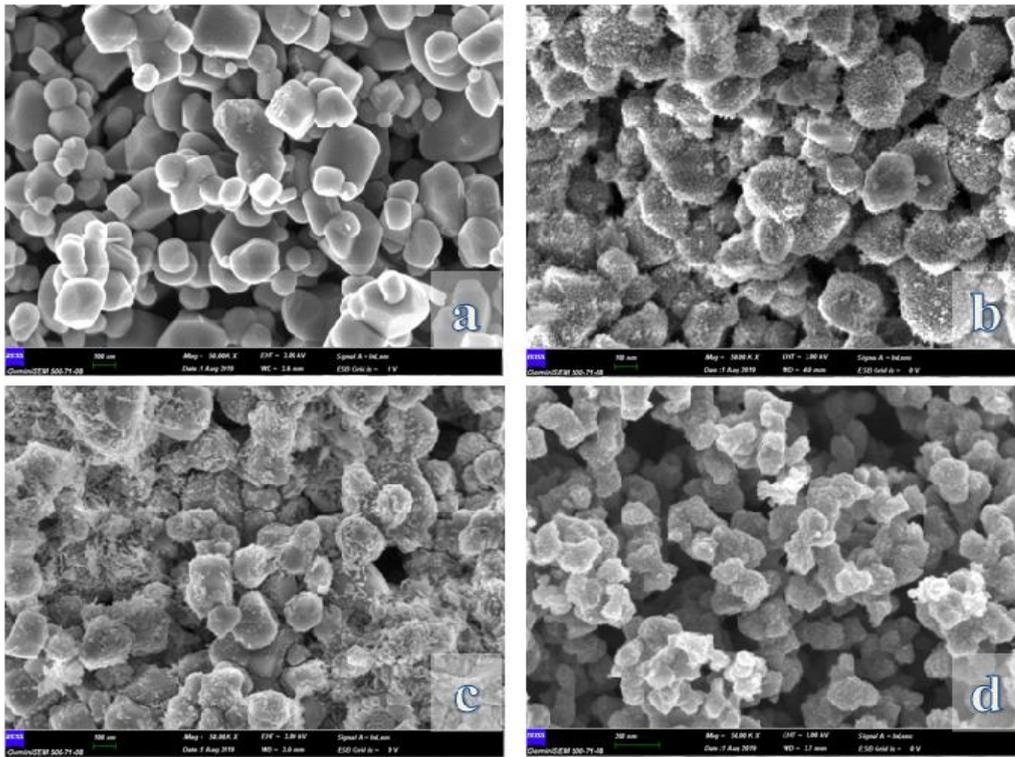
Figure 4. FESEM images of a) pure TiO<sub>2</sub> b) TiO<sub>2</sub>+ sodium dodecyl sulfate (SDS) c) TiO<sub>2</sub>+cetyl trimethyl ammonium bromide (CTAB), and d) TiO<sub>2</sub>+nonionic (TritonX-100).
