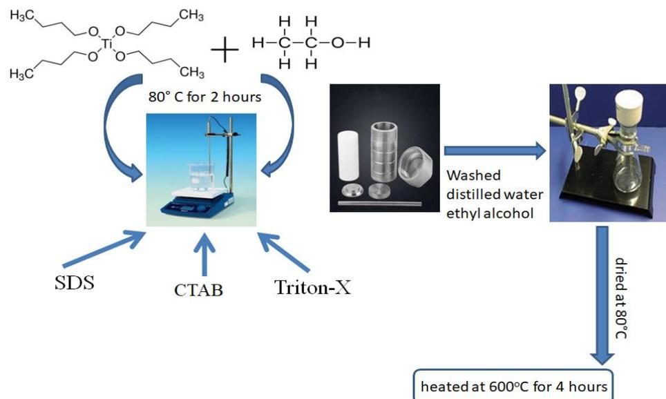
Figure 1. Schematic illustration of TiO<sub>2</sub> synthesis by surfactant assisted hydrothermal method.
