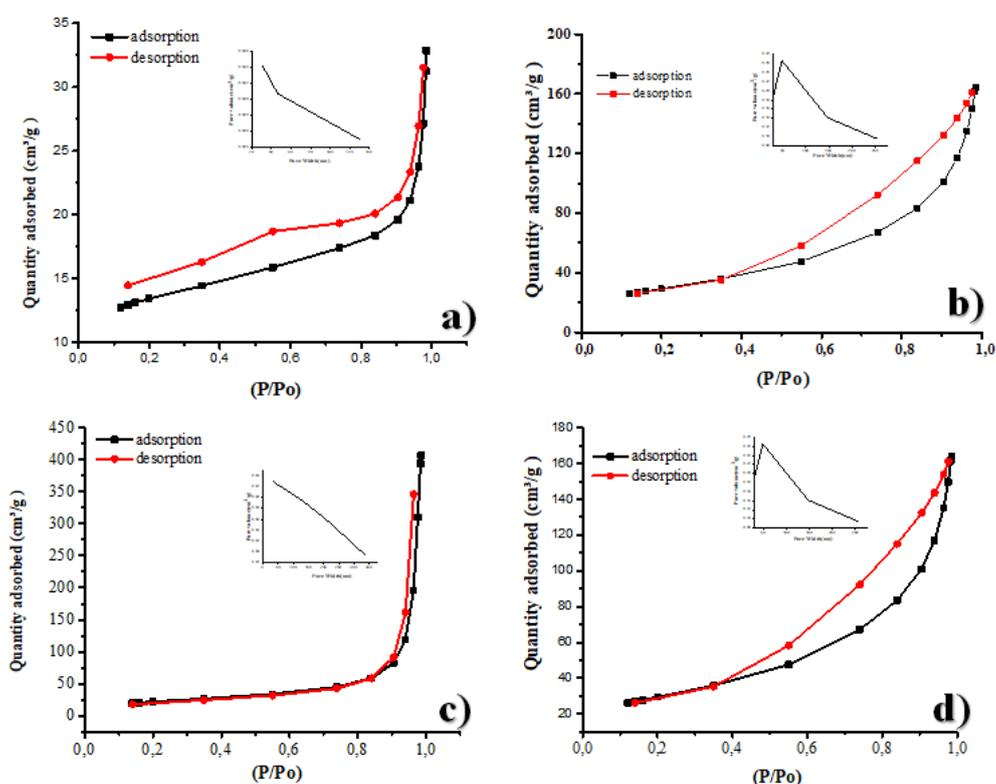
Figure 6. N<sub>2</sub> adsorption/desorption isotherms and pore size distribution of a) pure TiO<sub>2</sub> b) TiO<sub>2</sub>+ sodium dodecyl sulfate (SDS) c) TiO<sub>2</sub>+cetyl trimethyl ammonium bromide (CTAB), and d) TiO<sub>2</sub>+nonionic (TritonX-100).
