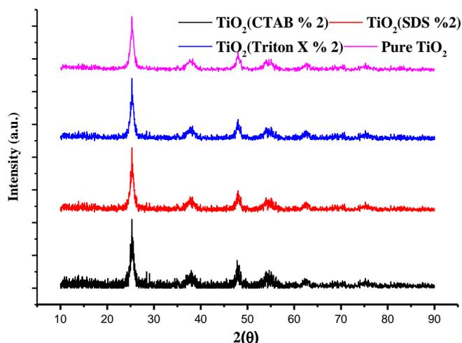
Figure 3. XRD patterns of the  $\text{TiO}_2$  materials with different surfactant additives a) sodium dodecyl sulfate (SDS) b) cetyl trimethyl ammonium bromide (CTAB), and c) nonionic (TritonX-100) in  $\text{TiO}_2$  suspensions.
