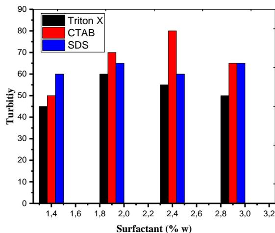
Figure 2. Turbidity of TiO<sub>2</sub> suspensions as a function of surfactant concentration.
