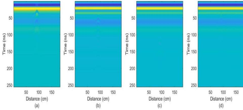
**Figure 2.** Raw data used for visual results: a) aluminum target, 1 cm burial depth and dry sand soil, b) aluminum target, 2 cm burial depth and wet sand soil, c) plastic target, 10 cm burial depth and dry clay soil, d) plastic target, 2 cm burial depth, dry loam soil.
