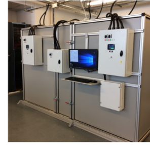
Figure 3. The calibrated hot box with the installed sample
