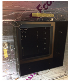
Figure 3. The calibrated hot box with the installed sample
