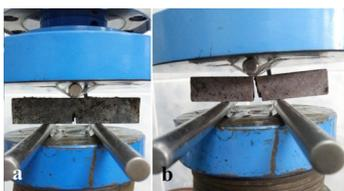
**Figure 2.** A three point flexural strength test specimen before loading (a) and after failure (b)
