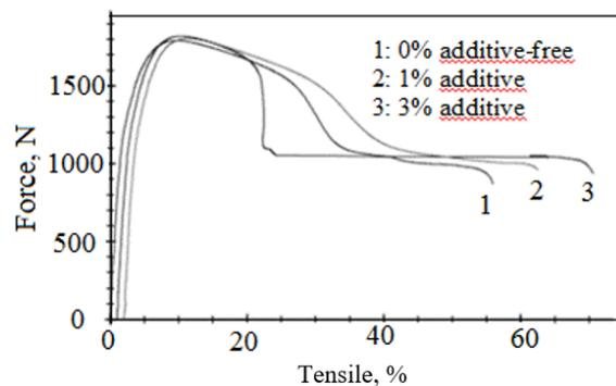
**Figure 6.** Tensile-Force Diagram applied on three different sample
