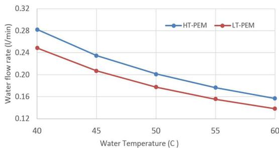
**Figure 4.** LT-PEMFC and HT-PEMFC cogeneration systems, water flowrate-water temperature graph
