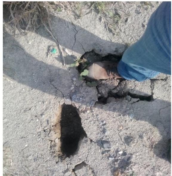
Figure 7. A photograph showing the very low soil bearing capacity of area-2
