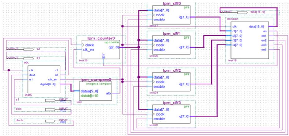
Figure 7. The receiver scheme implemented on FPGA board.
