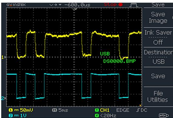
Figure 8. Modulated (blue line) and received (yellow line) signals for low frequency.
