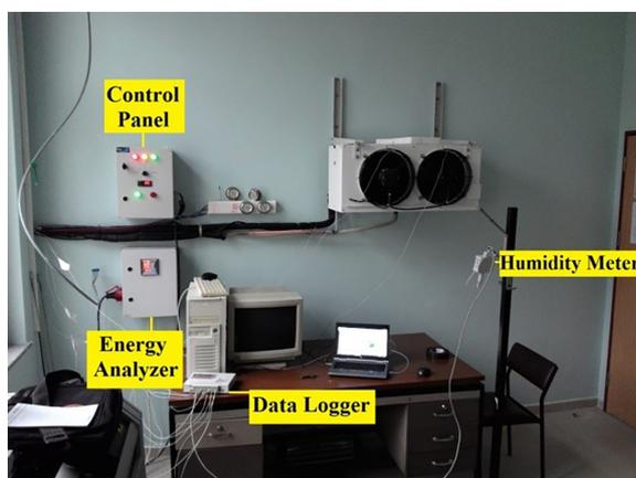
Figure 2. Indoor unit of the heat pump
