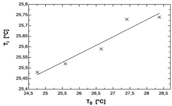
**Figure 9.** Change of indoor air temperature as a function of outdoor air temperature
