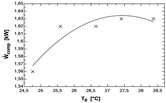
**Figure 5.** Variation of compressor power consumption as a function of outdoor air temperature
