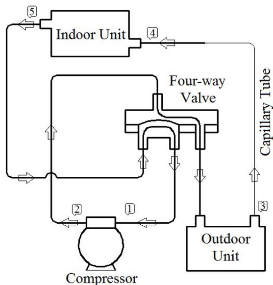
Figure 1. Heat pump cycle in cooling mode
