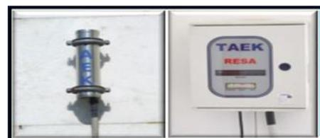
Figure 4: RESA detector- counter and control center, TAEK [20]
