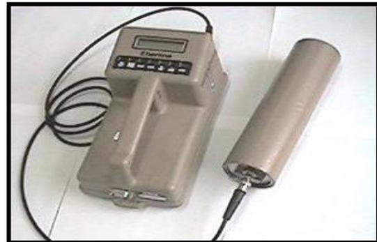
**Figure 2:** ESP-2 Rate meter and SPA-6 scintillation detector; Eberline [18]
