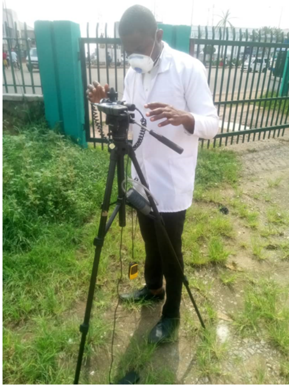
Figure 2. Measurement and calibration exercise of PM Real-time Dust Monitor (Casella, Bedford, UK).
