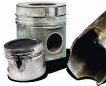
Figure 2.6. Damage caused by exhaust brake malfunctions
