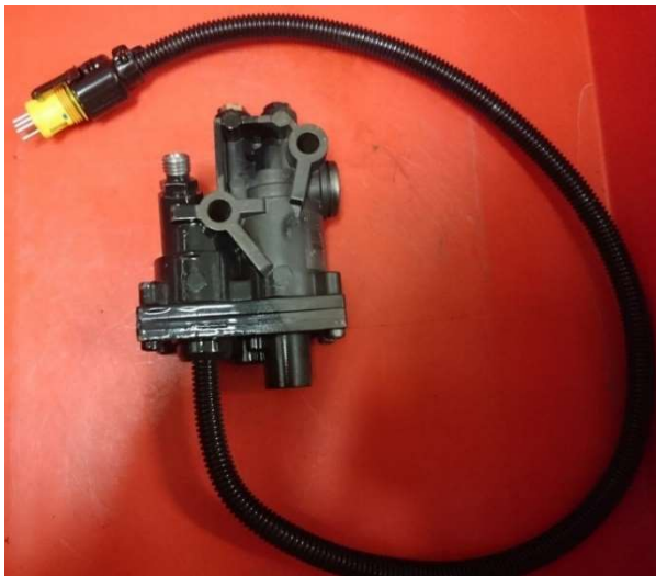
Figure 2.7. Exhaust brake valve used in MAN vehicles
