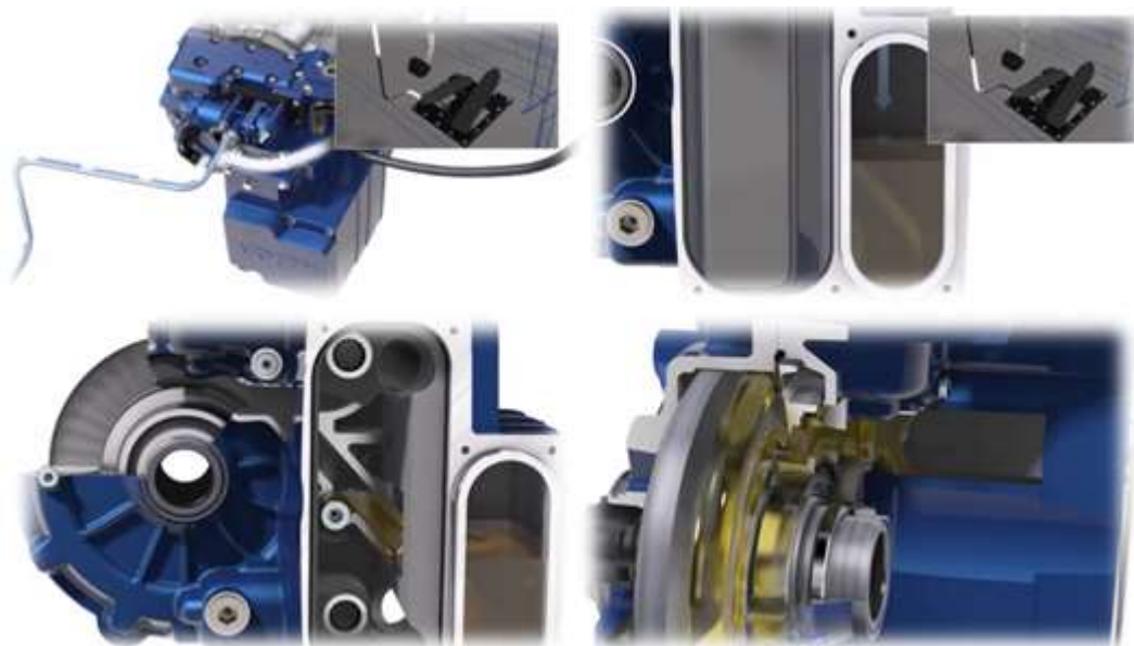
Figure 3.2. Pressing the oil into the system
