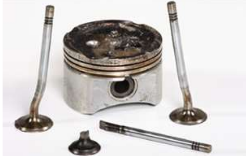
Figure 2.6. Damage caused by exhaust brake malfunctions
