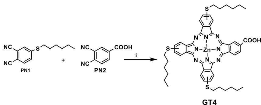
**Scheme 1.** The synthetic pathway of GT4 (i) ZnCl<sub>2</sub>, DMF (dimethylformamide), (1,8-diazabicyclo [5.4.0] undec-7-ene) (DBU), 160 °C.
