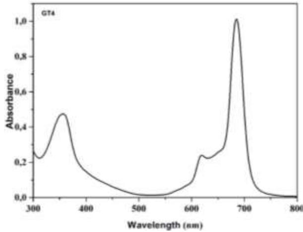
**Fig. 1** Absorption spectra of **GT4** in THF ( $1 \times 10^{-5}$  M).
