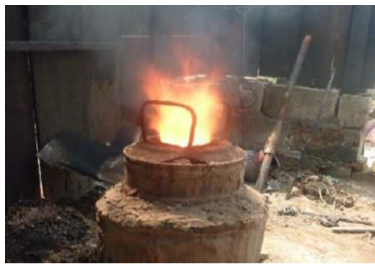
Figure 1. Melting of copper alloy in the crucible furnace
