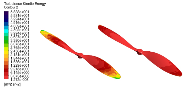
Figure 6. Turbulent kinetic energy contours of 6000-RPM (left) and 3000-RPM (right) at 2.4 m/s airspeed
