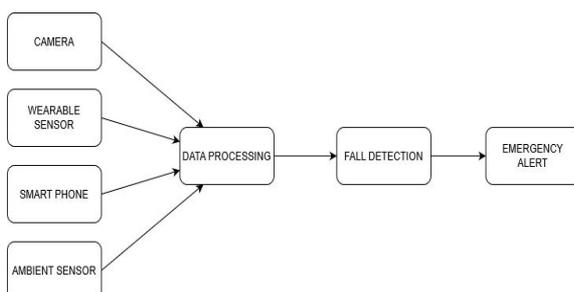
**Figure 1.** General block diagram of fall detection systems
