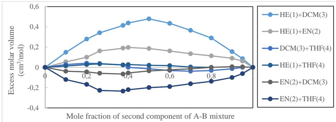
**Figure 1.** For the three binary systems, experimental values of excess molar volume as a function of n-hexanol molar fraction: symbols apply to the experimental data while the lines reflect the results of the ternary Hexanol + Ethanenitrile + Dichloromethane + tetrahydrofuran quaternary method determined from the Redlich-Kister-Muggianu formalism.
