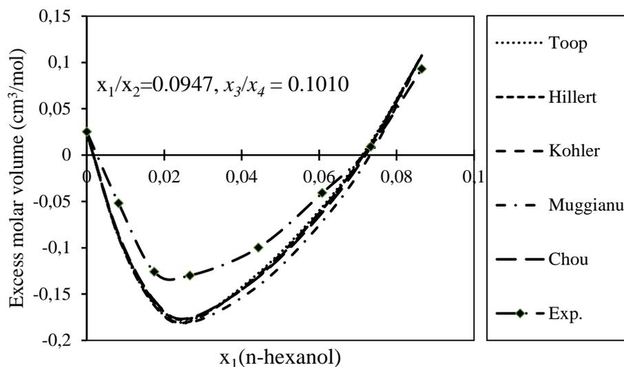
**Figure 4.** Comparison of the traditional models, Chou model and experimental data of excess molar volume for the section  $x_1/x_2 = 0.0947$ ;  $x_3/x_4 = 0.1010$  in the quaternary Hexanol + Ethanenitrile + Dichloromethane + tetrahydrofuran quaternary system.
