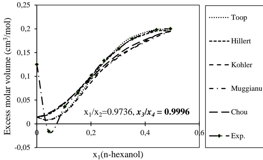
**Figure 6.** Comparison of the traditional models, Chou model and experimental data of excess molar volume for the section  $x_1/x_2 = 0.9736$ ;  $x_3/x_4 = 0.9996$  in the quaternary Hexanol + Ethanenitrile + Dichloromethane + tetrahydrofuran quaternary system.
