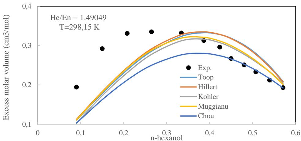
**Figure 2.** Comparison of the traditional models, Chou model and experimental data associated with the excess molar volume for the section  $x_1/x_2 = 1.49049$  in the ternary Hexanol + Ethanenitrile + Dichloromethane.
