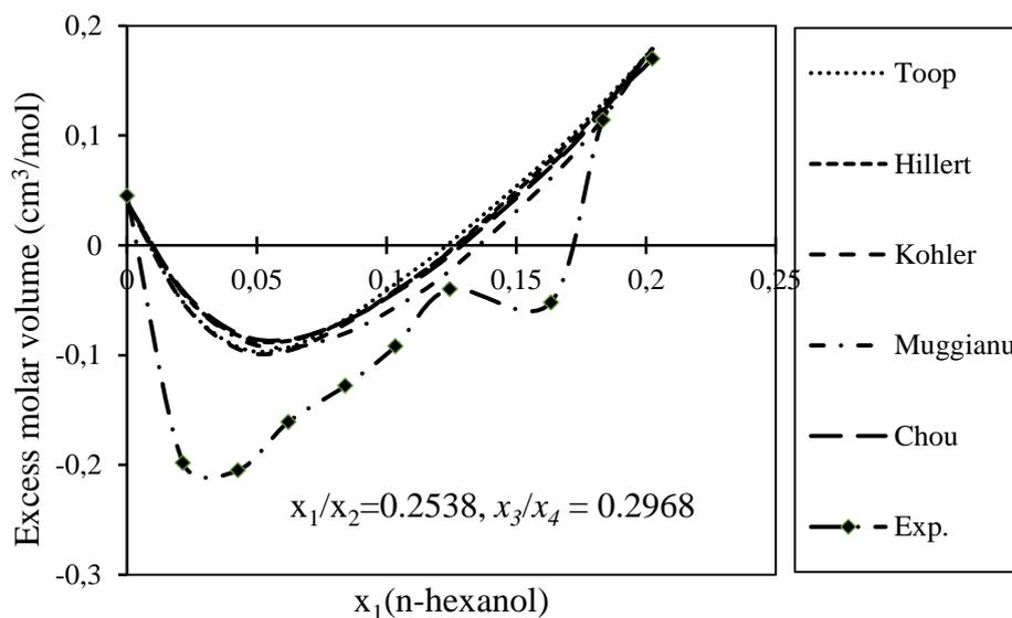
**Figure 5.** Comparison of the traditional models, Chou model and experimental data of excess molar volume for the section  $x_1/x_2 = 0.2538$ ;  $x_3/x_4 = 0.2968$  in the quaternary Hexanol + Ethanenitrile + Dichloromethane + tetrahydrofuran quaternary system.
