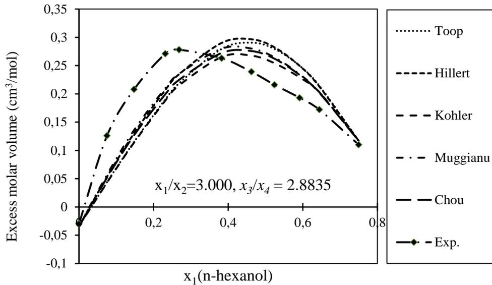
**Figure 7.** Comparison of the traditional models, Chou model and experimental data of excess molar volume for  $x_1/x_2 = 3.0000$ ;  $x_3/x_4 = 2.8835$  in the quaternary Hexanol + Ethanenitrile + Dichloromethane + tetrahydrofuran quaternary system.
