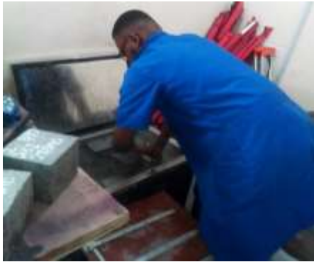
Figure 2. Curing of concrete cubes
