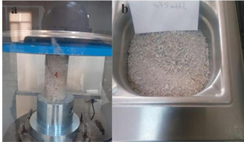
**Figure 2.** Experimental studies (Sample prepared for uniaxial pressure experiment and  $\text{Na}_2\text{SO}_4$  experiment)
