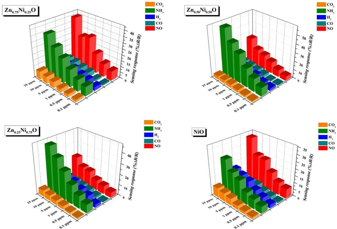
**Figure 7.** The Selectivity of the Sensors Exposed to NO, CO, NH<sub>3</sub>, H<sub>2</sub> and CO<sub>2</sub> Gases for Different Gas Concentrations at 85 °C
