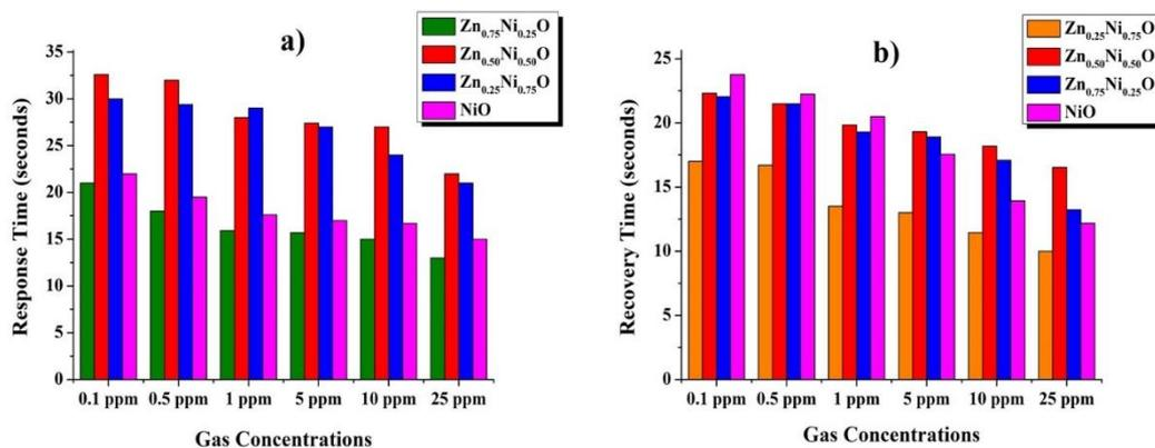
Figure 6. The Response and Recovery Times of Zn<sub>1-x</sub>Ni<sub>x</sub>O for 20 ppb-25 ppm
