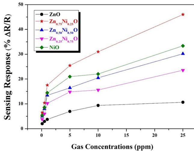
Figure 5. The Sensing Responses of Zn<sub>1-x</sub>Ni<sub>x</sub>O for Different Gas Concentrations from 100 ppb to 25 ppm at 85 °C
