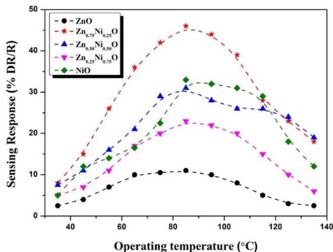
**Figure 3.** The Sensing Responses of the Sensors versus Operating Temperature at Constant 25 ppm NO Gas Concentrations
