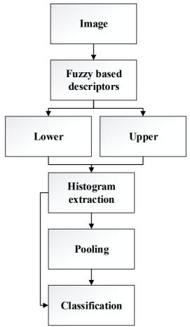
Figure 7. Block diagram of the proposed fuzzy architecture.
