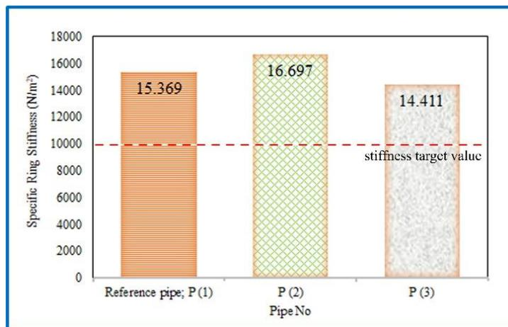
Figure 6 Change of the stiffness values according to the pipe type
