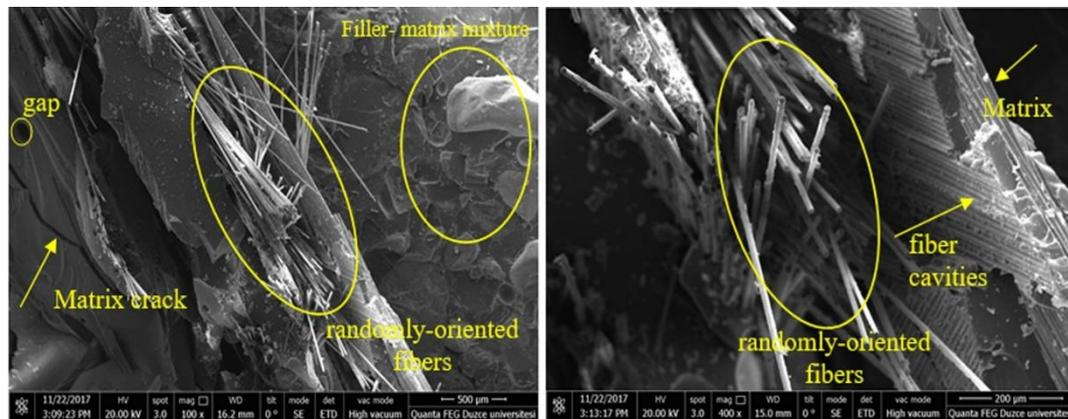
Figure 9 SEM images in the core region of F0.8 grain distributed GRP pipes
