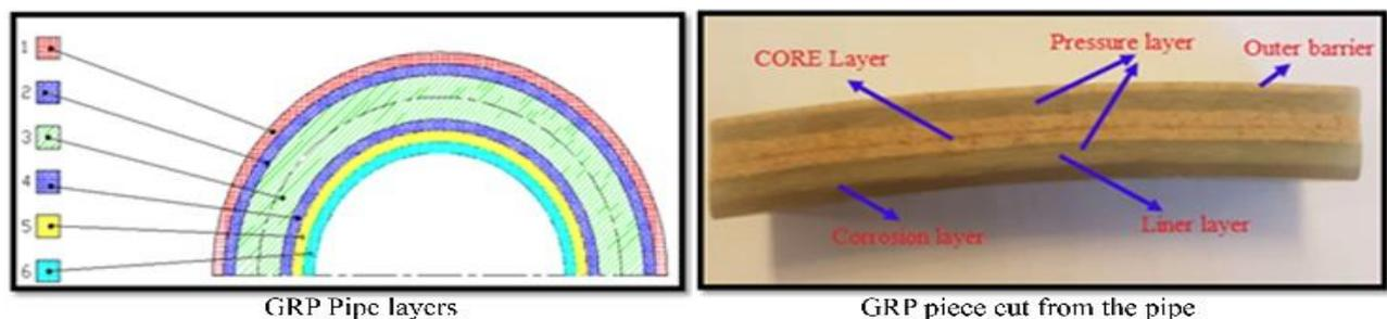
Figure 3 The schematic representation of the pipe section produced by the CC method and a visual of the part cut from the produced pipes
