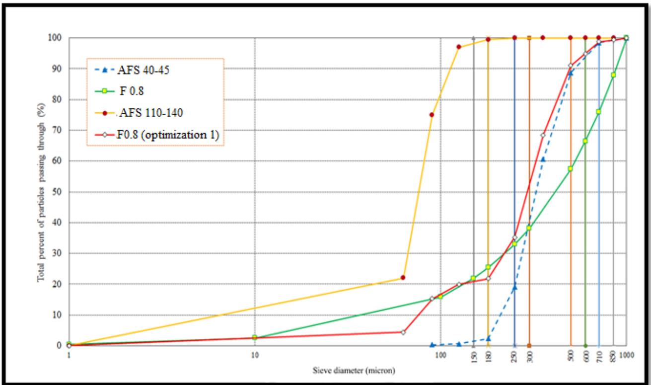
Figure 1 Different filler grain size distribution graphics used in the study
