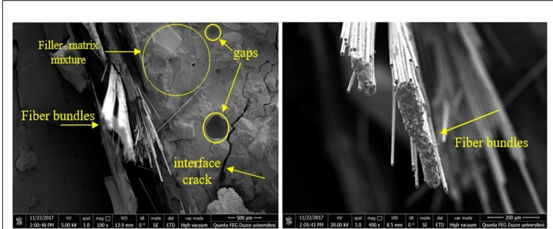
Figure 8 SEM images in the core region of AFS 40-45 grain distributed GRP pipes
