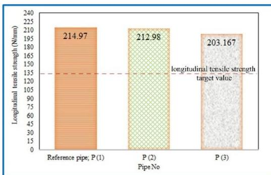
Figure 7 Change of the LTS values according to the pipe type
