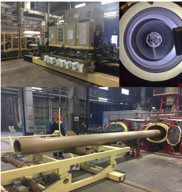
Figure 2 GRP pipe production process by the CC method
