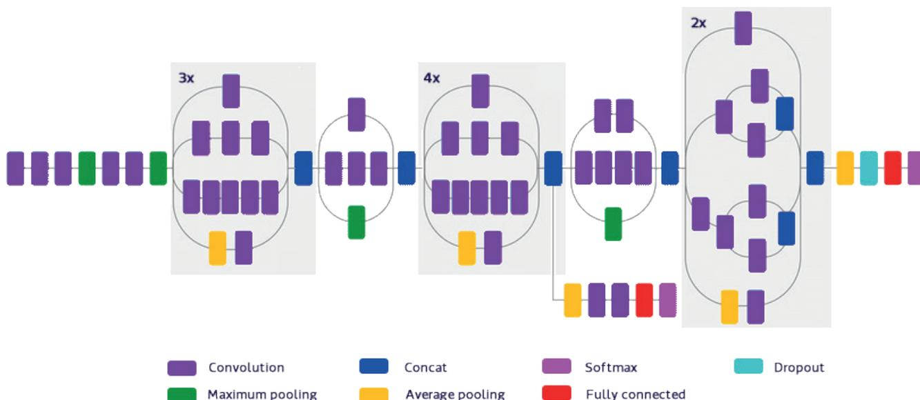
Figure 8. Structure of Inception v3 model (Agrawat and Raval 2018)
