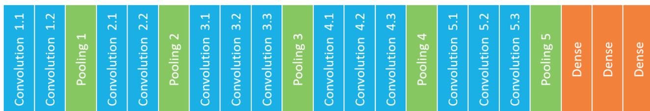
Figure 6. Structure of VGG-16 model
