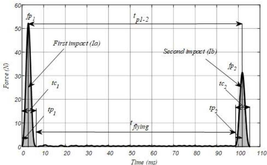
Figure 2. Sample graph for impact force-time and measured nondestructive impact parameters
