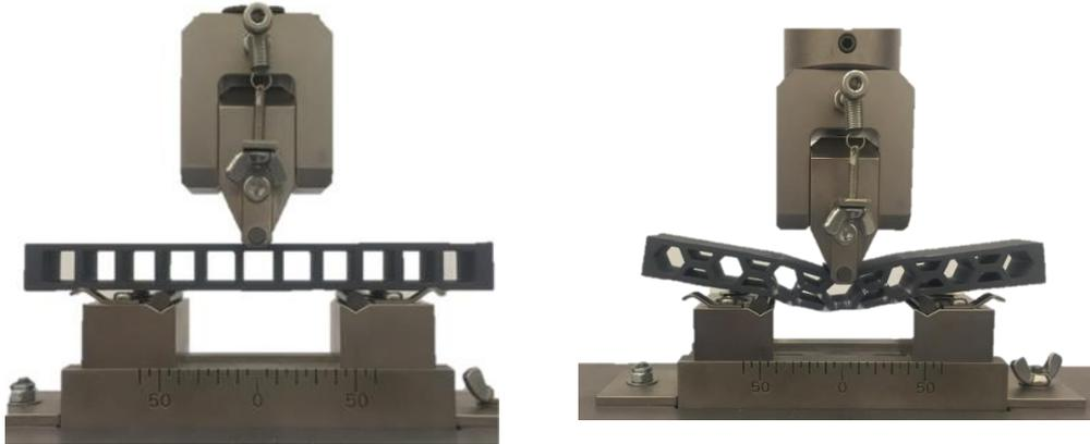
**Figure 2.** Three-point bending test configurations of 3D printed structures.
