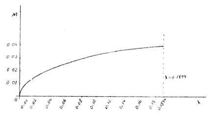
This shows that M increases as  $\lambda$  or the frequency n of the periodic motion of the cylinder increases, and it reaches the value 0.0401 when  $\lambda=0.1894$ . This value of  $\lambda$  sorresponds to  $n=1270/{\rm sec.}$  Hence when the frequency of the cylinderis 1270 per second the amplitude of the diverging waves at a point 100 metres distant from the axis of the cylinder is 0.0401  $\delta_0$ .
