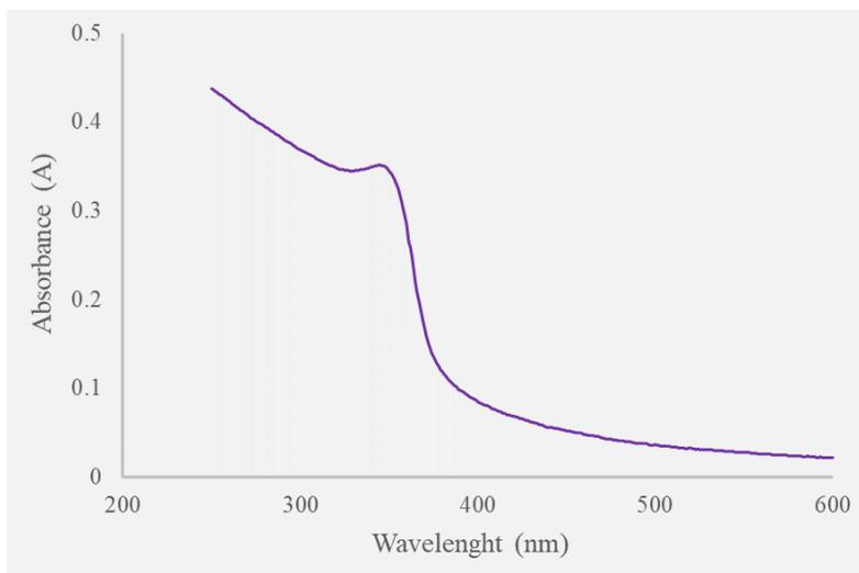
**Figure 2:** Uv-Visible spectrum of ZnO NPs
