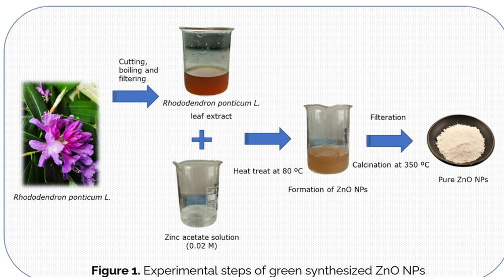
**Figure 1.** Experimental steps of green synthesized ZnO NPs
