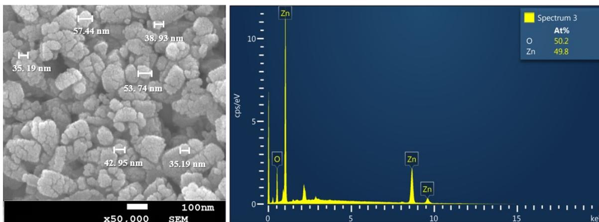
**Figure 3:** SEM images of ZnO NPs with EDX spectrum
