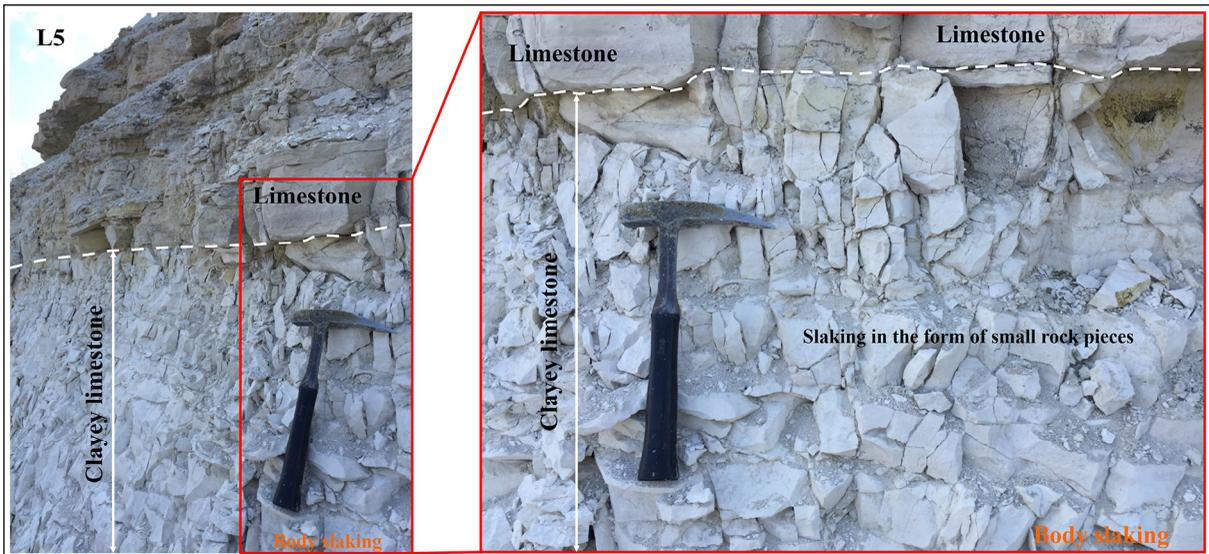
Figure 10- A typical example of the body slaking behaviour in clayey limestones in the form of small rock pieces in atmospheric conditions (L5).
