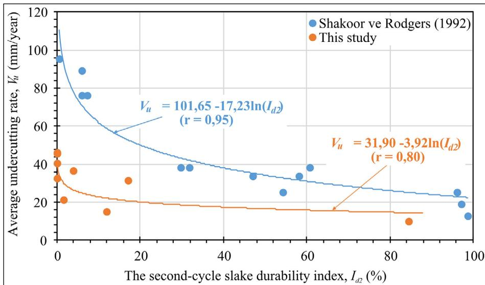
Figure 9- The relationships between average undercutting rate values and second-cycle slake durability index values obtained in this study and studies carried out by Shakoor and Rodgers (1992).
