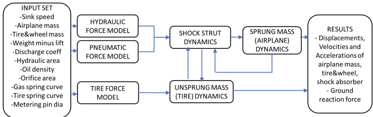
**Figure 2.** Flowchart of landing gear simulation (adopted from [3]).
