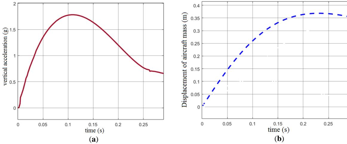
**Figure 9.** Optimized geometry (a) vertical acceleration (g) vs time (s); (b) displacement of aircraft mass (m) vs time (s)
