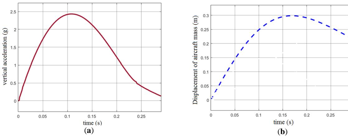
Figure 8. Initial unoptimized geometry (a) vertical acceleration (g) vs time (s); (b) displacement of aircraft mass (m) vs time (s)
