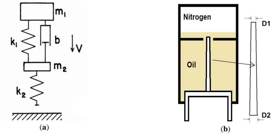
**Figure 1.** (a) Mass-spring-damper model for landing gear; (b) Shock absorber cross section and metering pin diameters.
