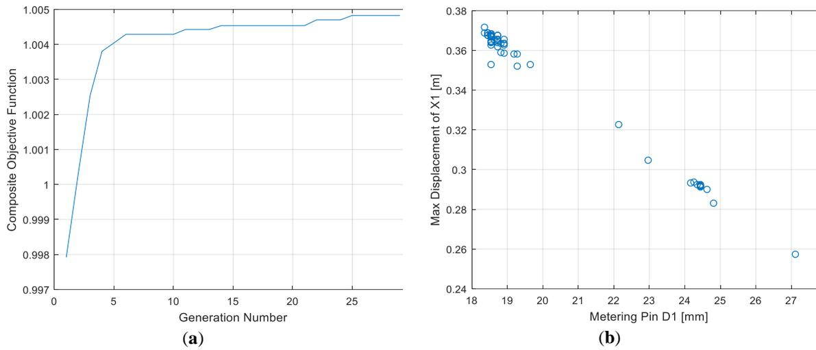
Figure 4. (a) Objective function vs. generations (iterations); (b) Displacement of aircraft mass vs. D1.
