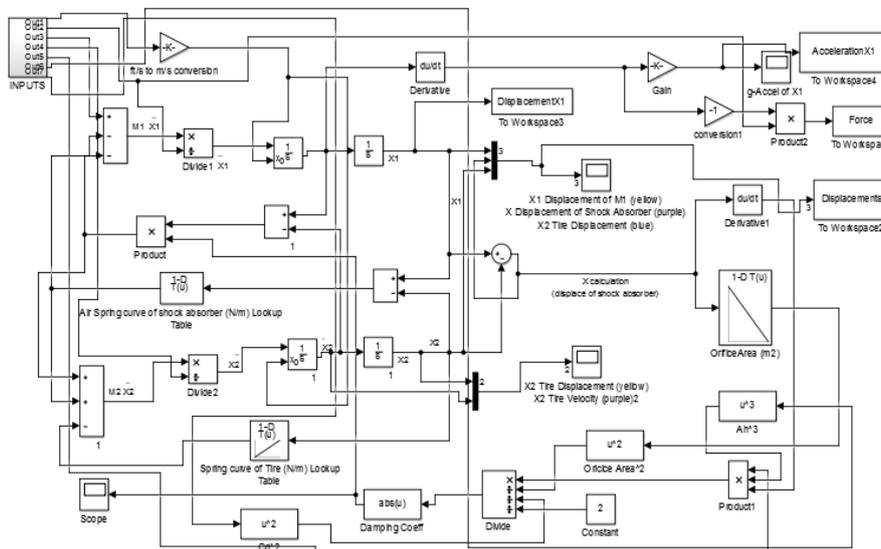
Figure 3. Simulink model of landing gear.
