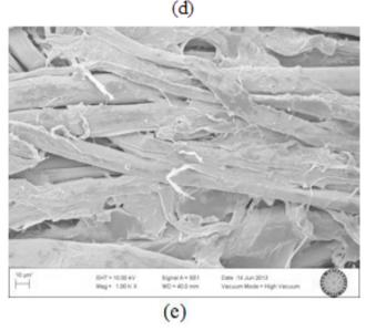
**Figure 1.** The SEM images of raw flax fabric (a), treated with oxygen plasma for 5 minutes (b), treated with oxygen plasma for 10 minutes (c), treated with nitrogen plasma for 5 minutes (d), treated with nitrogen plasma for 10 minutes (e)
