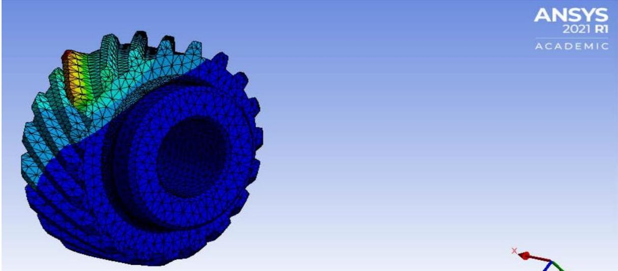
**Figure 8.** Deformations in helical gear wheels.
