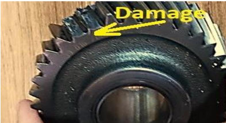
**Figure 4.** The damaged helical gear wheel.
