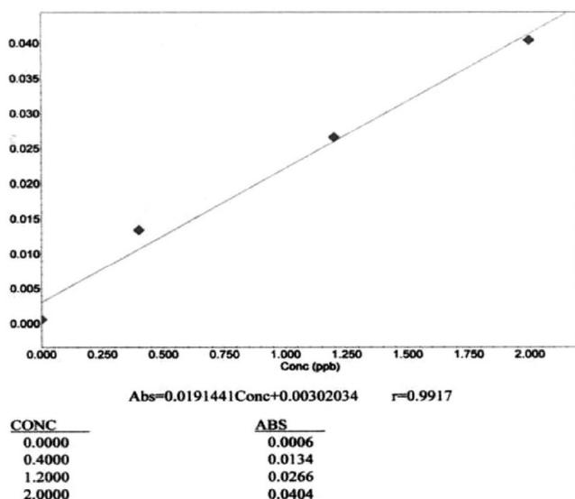
Figure 3. Manganese calibration curve
