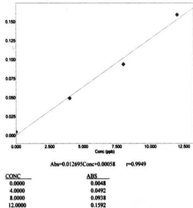
Figure 1. Lead calibration curve
