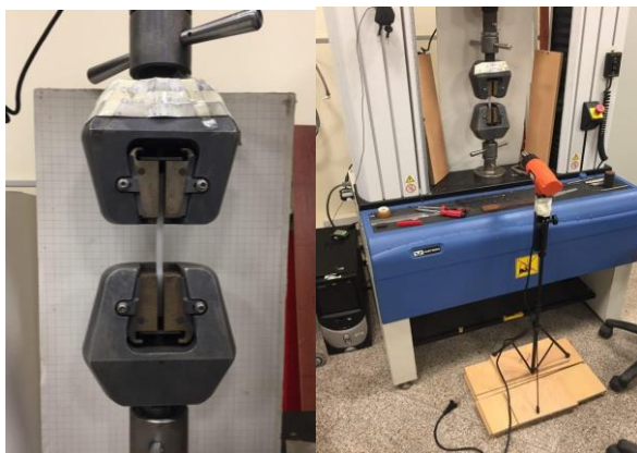
Figure 6. Test coupon inside Instron machine (Left) and the machine with a heat gun pointing at the coupon (Right)
