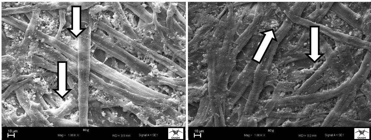
Figure 4. SEM images of recycled paper and base paper, Left: Base paper, Right: recycled paper
