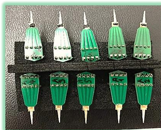
Figure 4. Image of new microelectrodes that were made ready for test after completing the fabrication.
